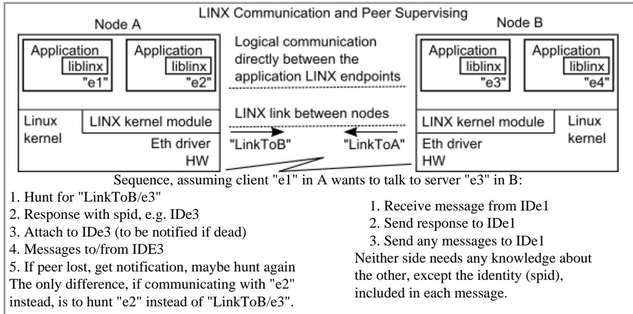
Communication is transparently routed across a series of nodes, if a series of link names are given before the endpoint name, e.g. "ToC/ToB/server".
