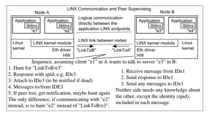
Communication is transparently routed across a series of nodes, if a series of link names are given before the endpoint name, e.g. "ToC/ToB/server".
