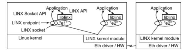
The LINX protocol, used by the LINX kernel module, has two main levels, RLNH and CM. RLNH is generic and handles logical LINX connections and supervision within and between nodes. CM provides a reliable transport. If the underlying transport is non-reliable, e.g. Ethernet, CM needs to provide reliability.
