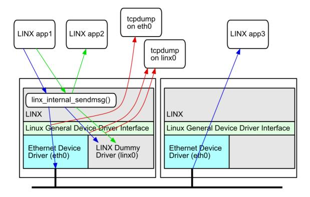
There is a feature in LINX to make the internal messages visible as well. This is done by duplicating all messages that are sent within LINX (linx\_internal\_sendmsg()) to a special dummy network driver called linx0. Since LINX 1.2, there are also patches for tcpdump and libpcap included in the release. These patches make tcpdump and libpcap understand the messages that are sent to linx0. Please note that there are only patches for tcpdump-3.9.4 and libpcap-0.9.4.
