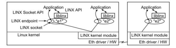
The LINX protocol, used by the LINX kernel module, has two main levels, RLNH and CM. RLNH is generic and handles logical LINX connections and supervision within and between nodes. CM provides a reliable transport. If the underlying transport is non-reliable, e.g. Ethernet, CM needs to provide reliability.
